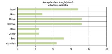
The tests have been conducted at  $20^{\circ}$ C on metal to metal joints, which have been hardened for 48 hours at  $20^{\circ}$ C.
